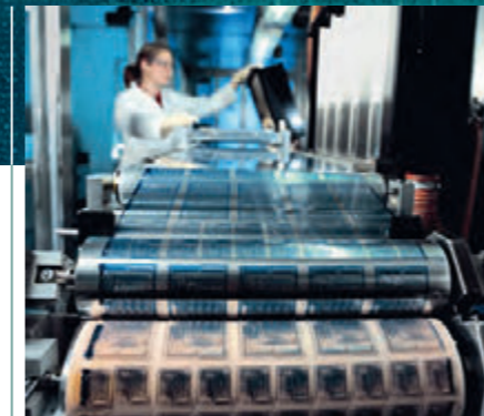
Printed electronics: RFID tags for PolyIC GmbH.
